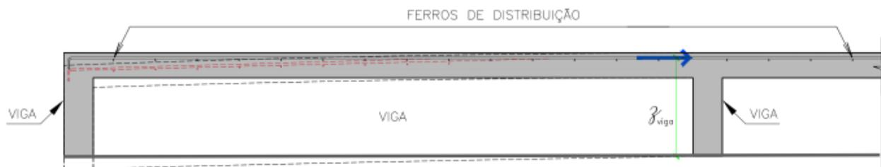
$Z_{laje} \lll Z_{viga} \Rightarrow$  COM VIGA TENDE A DEFORMAR MENOS, EXIGIR MENOS AÇO, ...
